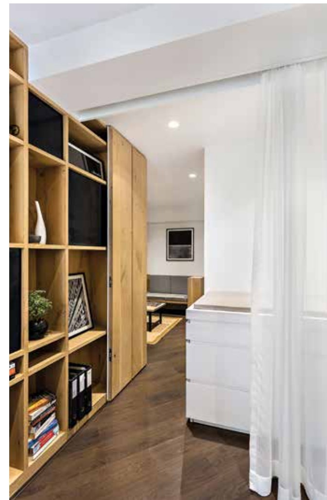
ABOVE LEFT The examination table can be hidden behind a sheer curtain in the consultation room. It was designed and crafted in-house and has built-in storage under it. It is a wooden structure, clad in inexpensive veneer and finished in matte white PU.
